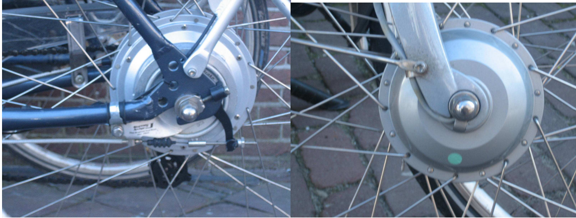
The hub motor in a rear wheel (left) and in a front wheel (right)
